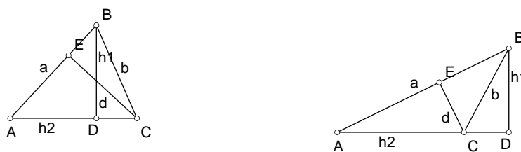
Figure 4: Automatic extension of the base line of a triangle. The point D is incident to the line AC , and the triangle side is given as a line with automatic endpoint clipping.
